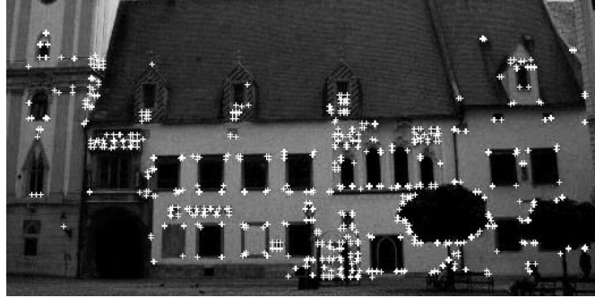
Figure 4.7. An example of the response of the Harris feature detector using 5 \times 5 integration window and parameter k = 0.04 .
